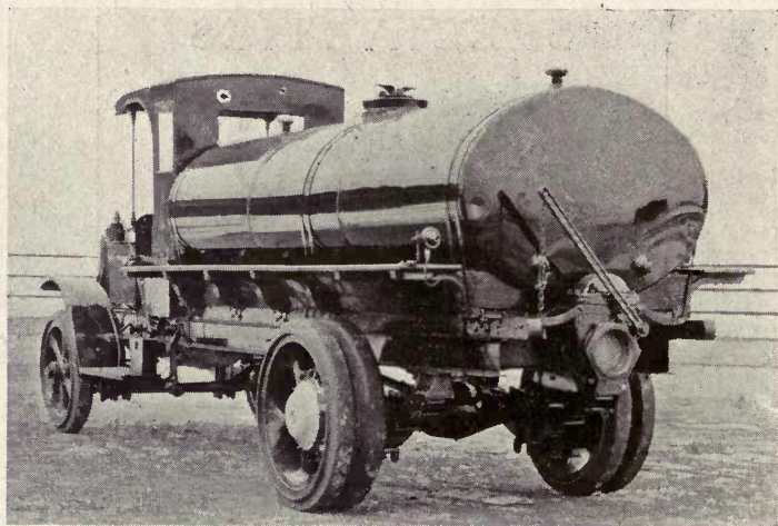
1,200-gallon fuel oil tank on 5-ton truck for the Gulf Refining Company—Heating coils, 2 cross sectional surge plates and one longitudinal surge plate, 14" manhole, 6" filler opening, two 2" McDonald vents, 8" piping and 8" gate valve.
