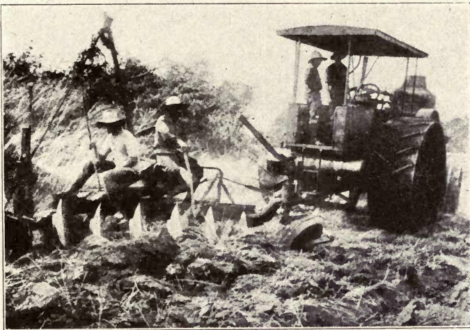
FIG. 88. Oil-Driven Tractor Pulling Plows on Sugar Estate. (Courtesy of Sinclair's Magazine.)
