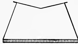
Fig. 10.—Bonnet with Concave Top and Crimped Bottom.
