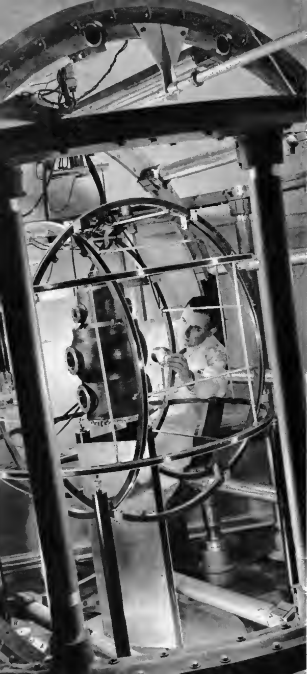
Gifford Scott collecting data in the large Helmholtz coils which cancel out the Earth's magnetic field.
