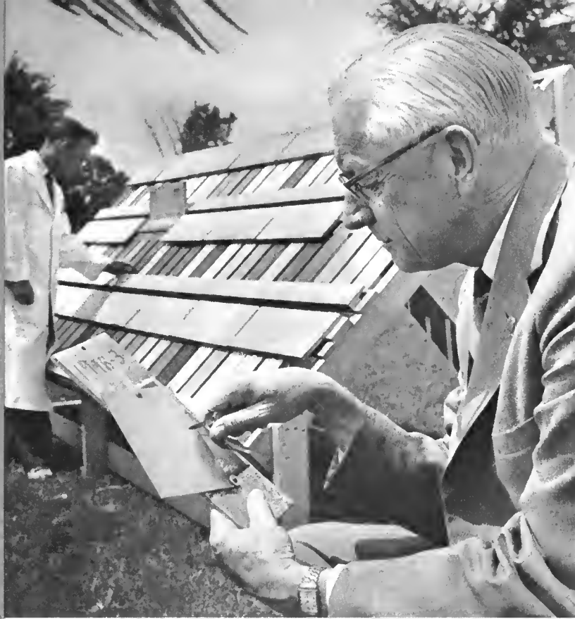
Ralph Wirshing inspects the original acrylic finished test panel after years of exposure at the GM Research Laboratories Florida Test Field.
