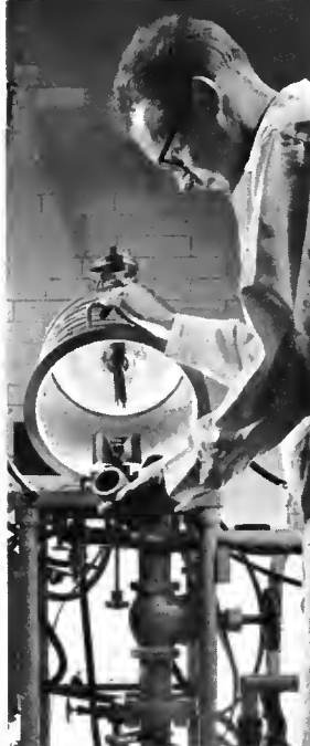
High temperature alloys are made in the special research furnace shown on the left and are tested in the unique heat and vibration fatigue apparatus on the right.
