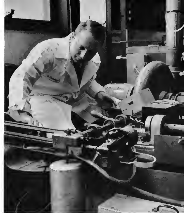
Carl Goodzeit adjusts the latest machine developed to test the seizure resistance of various bearing metals.
