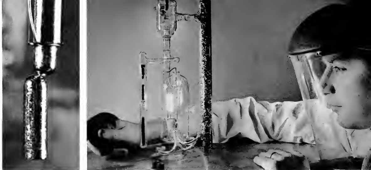
Carl Goodzeit bringing together the two specimens of polycrystalline copper (shown on the left) to determine their adhesion properties.
