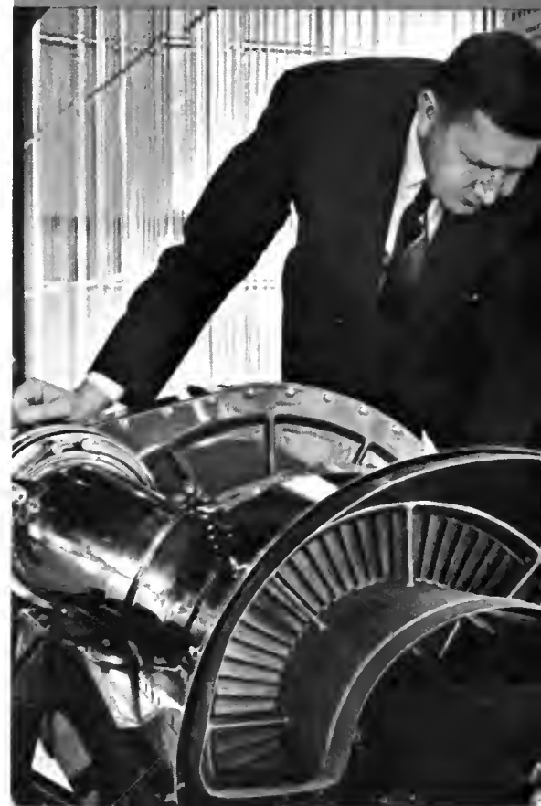
William Turunen and the Whirlfire gas turbine installed in Firebird I.
