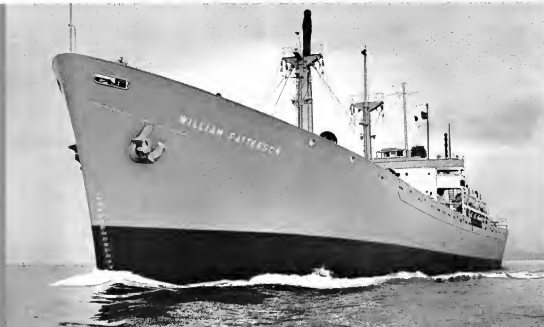
Six free-piston gasifiers produce over 6,000 horsepower to propel the William Patterson.
