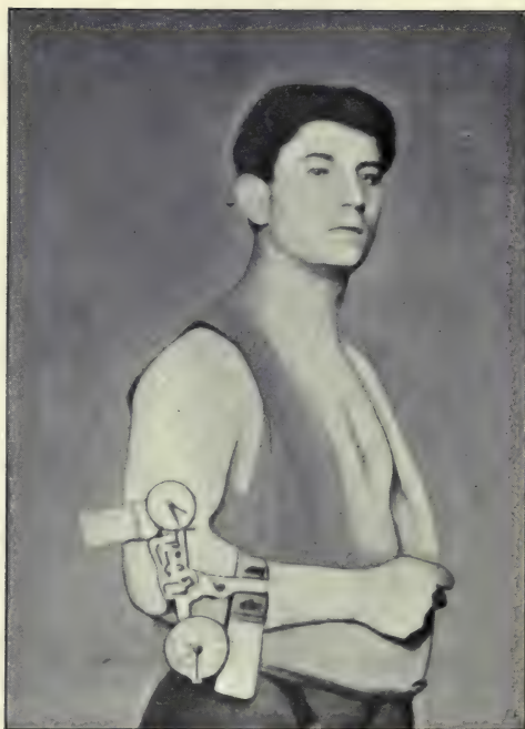
FIG. 6.—Arthrodynamometer fixed for measuring amount of movement of Elbow joint.
