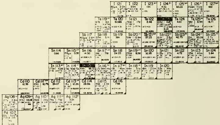
Figure III.B-1. Iodine spallation products produced at various proton bombarding energies. All products shown have a production cross section greater than 10 mb. Although more products are formed at higher energies, the total cross section remains nearly constant, ~1260 mb. The segments shown are from the Chart of Nuclides (Goldman, 1966).
