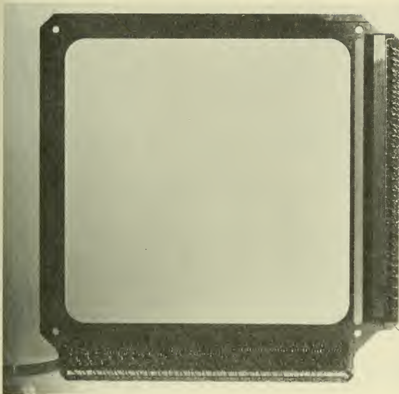
Figure IV.C-2. Photograph of a single wire grid spark-chamber module with two planes of 200 parallel wires. The direction of the wires in one plane is orthogonal to that in the opposite plane. Each wire is terminated through a ferrite core.
