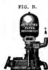
This Ram, whilst worked by a stream of impure water, will pump clear water from a well or spring.
