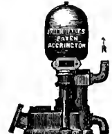
FIG. B.—This Ram, whilst worked by a stream of impure water, will pump clean water from a well or spring.
