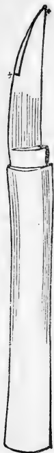
Fig. 34 .—Grafting Knife, with the portion of the back of the blade from + to + ground to a cutting edge, so as to make it serve also for a budding knife.
