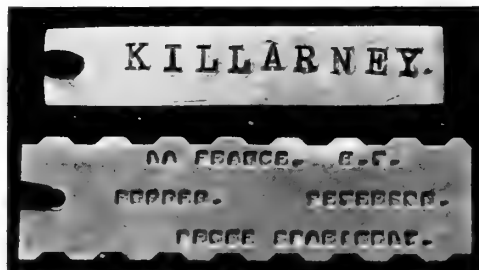
How much easier to read is the upper label made of aluminum with cut-in letters
