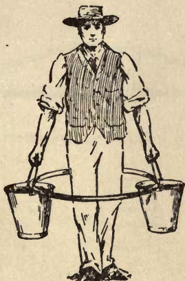
Fig. XIV.—The ring , for carrying two pails of water, with less exertion than if carried by the arms alone.
