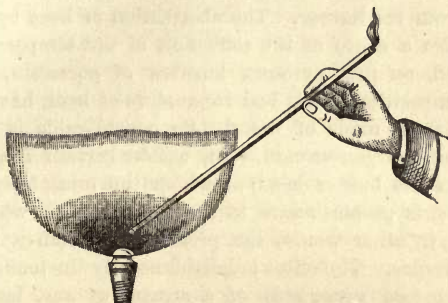
FIG. 4.—SHOWING THE TWO ZONES OF THE FLAME, AND THE METHOD OF DEMONSTRATING THE PRESENCE OF UNBURNT GAS IN THE FLAME.
