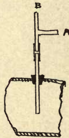
FIG. 15.—Method of supplying from large main.
