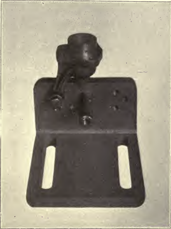
FIG. 114.—EXHAUST VALVE IN POSITION FOR DRILLING SCREW HOLES.
