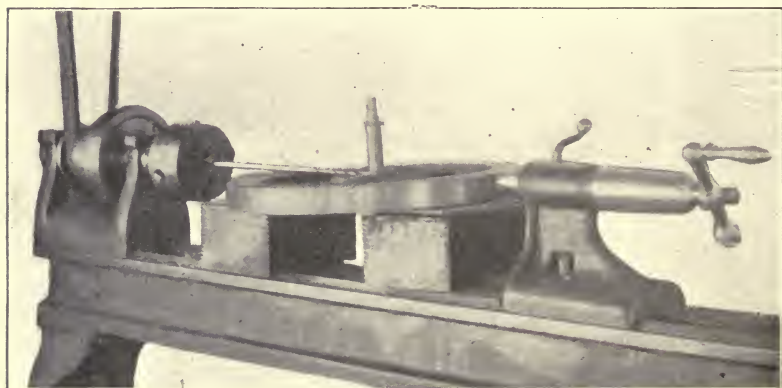
FIG. 95.—DRILLING FLY-WHEEL AND SHAFT FOR PIN.
