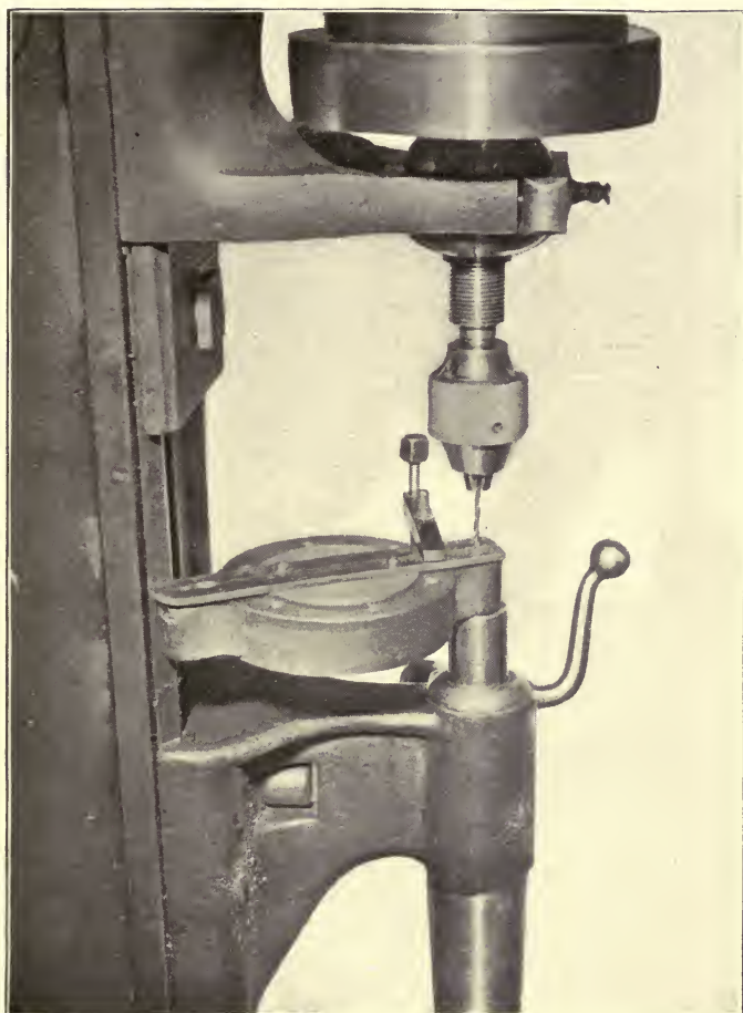
FIG. 52.—DRILLING CYLINDER COLLAR FOR SIDE RODS. DRILLING JIG IN POSITION ON COLLAR.
