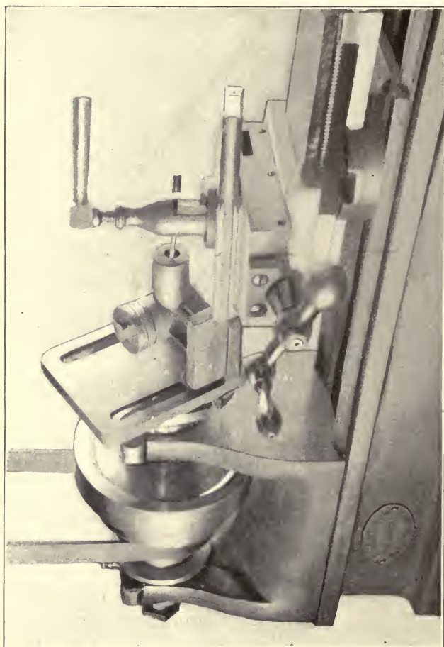
FIG. 76.—BORING MAIN BEARING FOR SIDE ROD.
