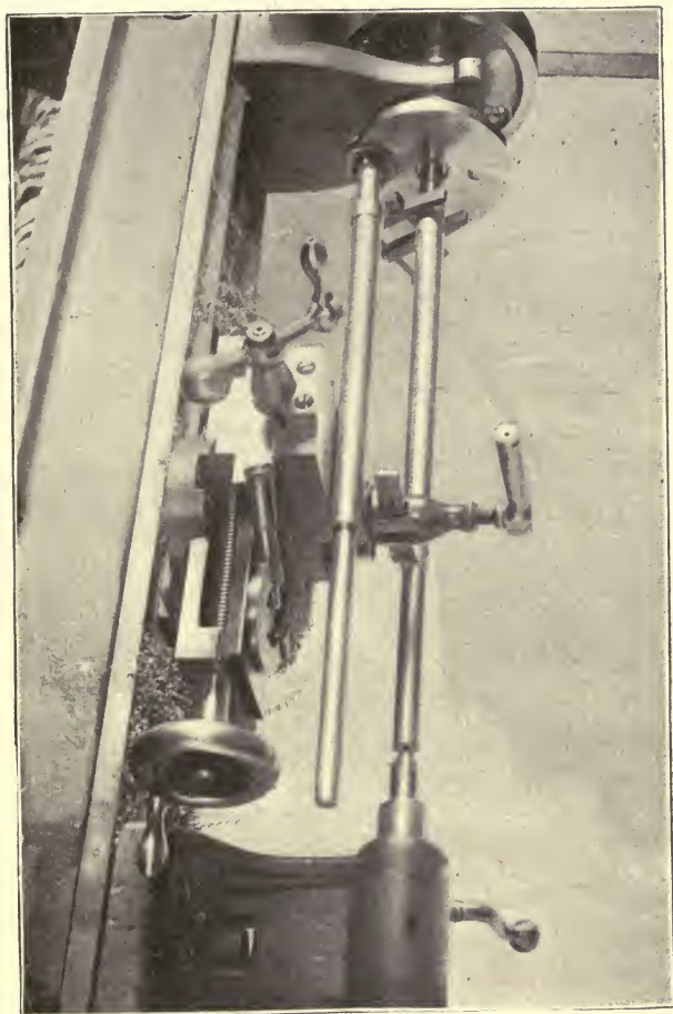
FIG. 85.—TURNING AND FINISHING SIDE RODS.
