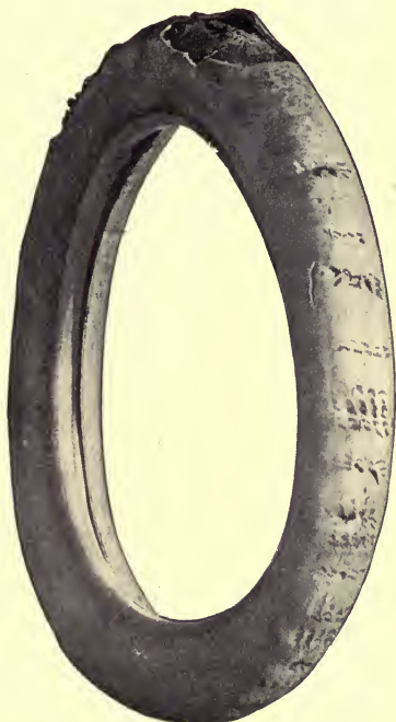
FIG. 250.—Tire injured by chains.
