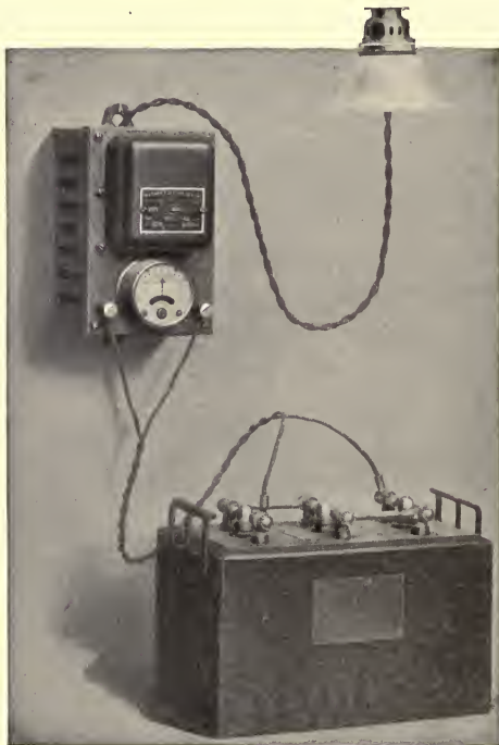
Fig. 211.—The Wagner rectifier charging a storage battery.
