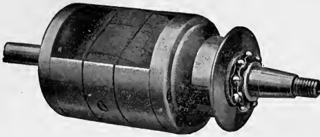
FIG. 179.—Armature of Remy Model P magneto.
