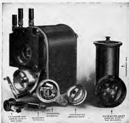
FIG. 182.—Connecticut magneto partially disassembled.
