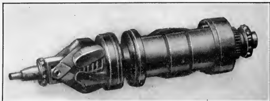
FIG. 184.—Eisemann armature with automatic spark advance mechanism.
