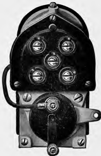
FIG. 178.—Distributor end view—Remy Model P magneto.
