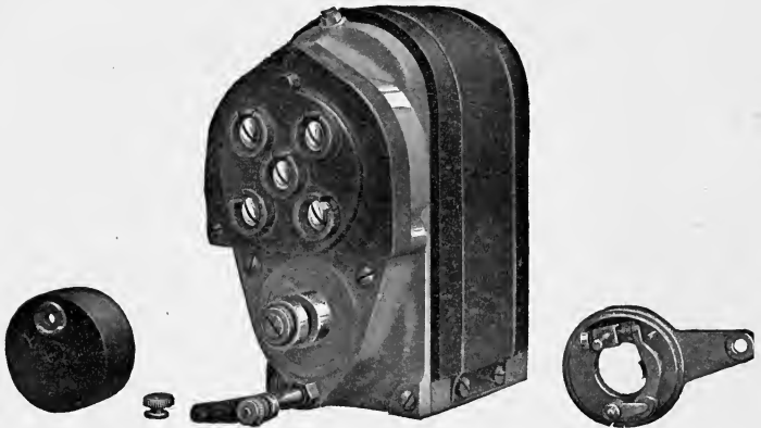
FIG. 180.—Remy Model P magneto—circuit breaker removed.
