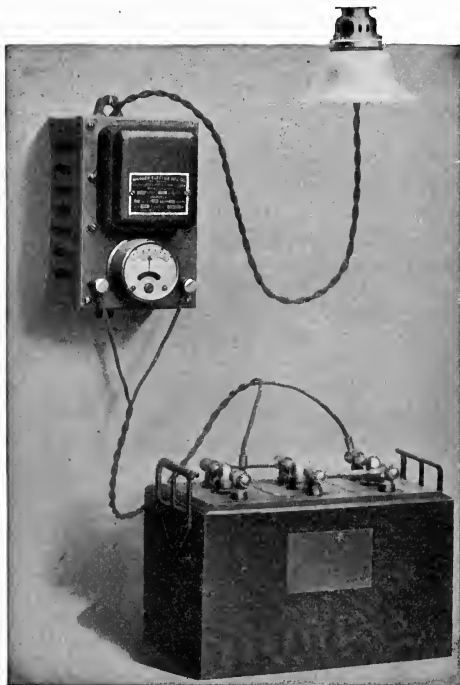
FIG. 211.—The Wagner rectifier charging a storage battery.
