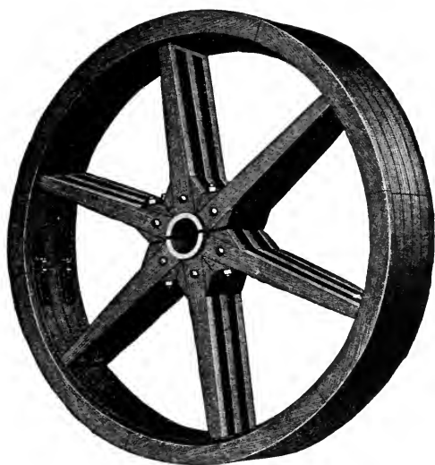
FIG. 97.—Construction of Split Wood Pulley.
