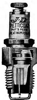
Fig. 44. Sectional View of a Spark Plug
