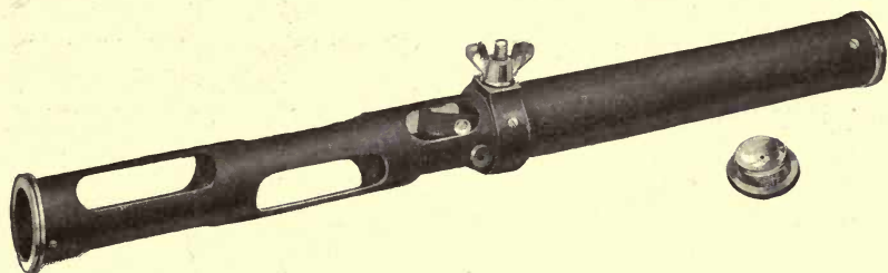
FIG. 79.—RECEIVING TUBE OF FOSTER'S FIXED FOCUS PYROMETER.
