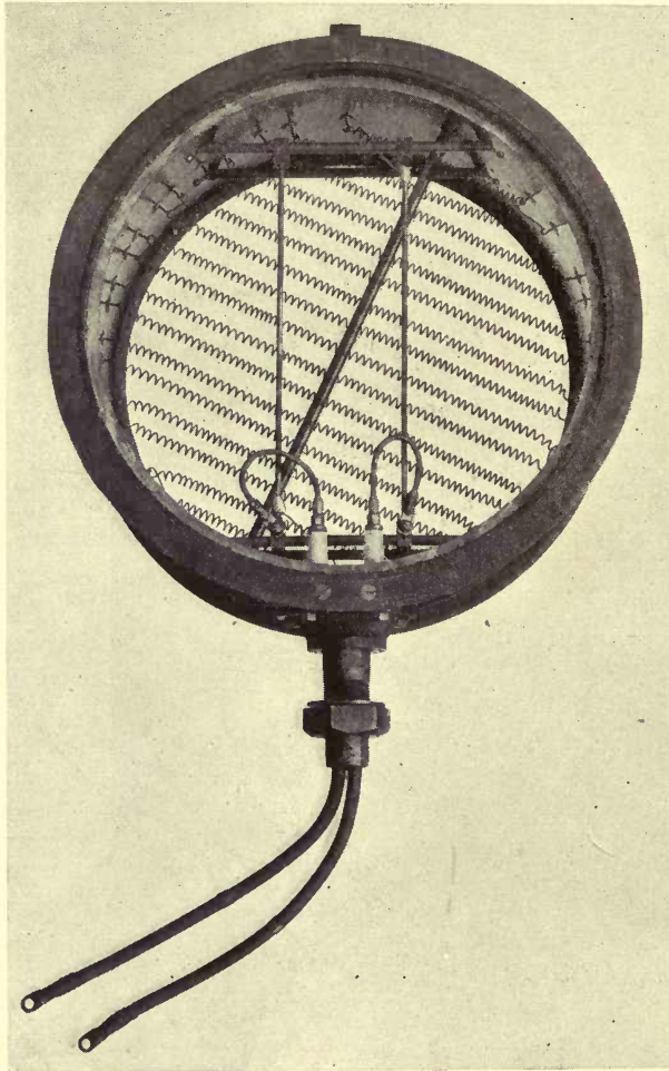
FIG. 164.—THERMOMETER FOR THOMAS METER.
