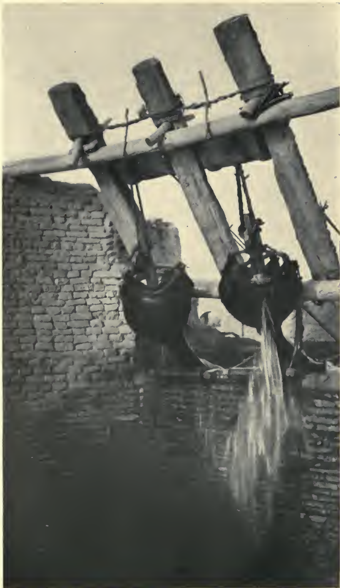
A Tigris Water Hoist at Work. The Leather Bags are Drawn up by Animals
