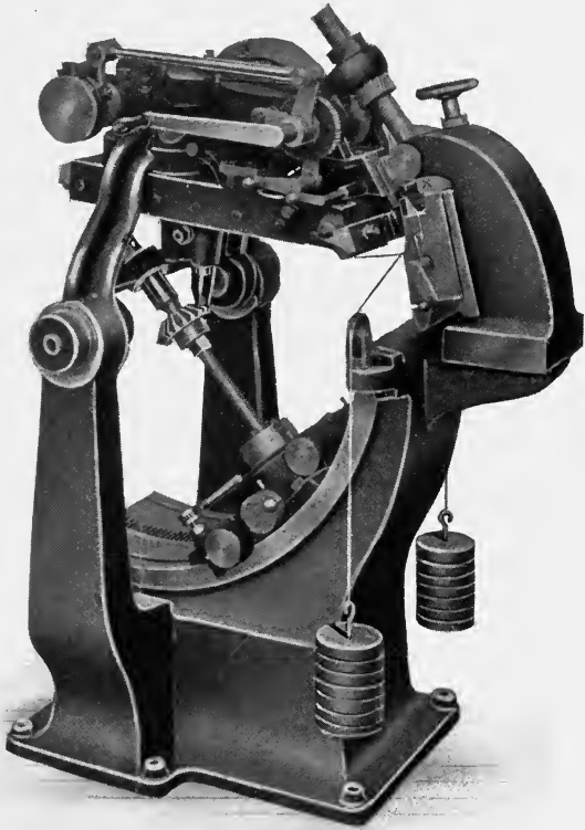
FIG. 184. A Hungarian Templet Bevel Gear Planer.
