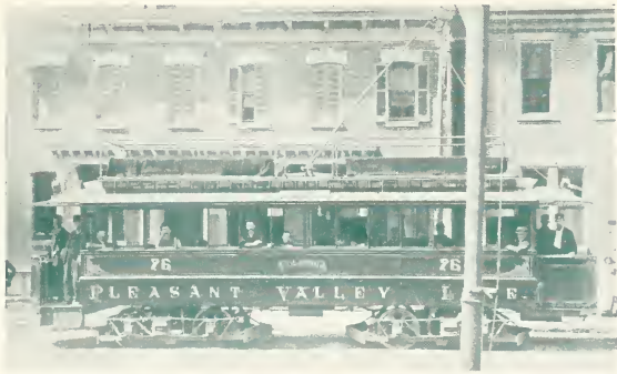
The first double truck electric street car in Pittsburgh, installed on the Pleasant Valley Line.
