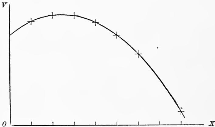
This is approximately parabolic in form and passes through the fixed point (0, 4.25). Therefore the relation between  $x$  and  $V$  may be expressed by the equation
