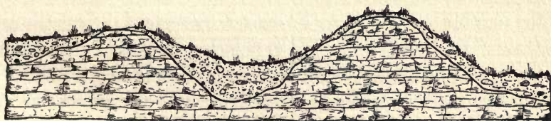
FIG. 33.—Diagrammatic section showing relation of drift to underlying rock where the drift is thin relative to the relief of the underlying rock.
