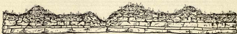
FIG. 47.—Section in a driftless area, showing relation of the mantle rock to the solid rock beneath.
