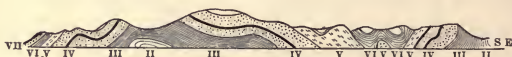
FIG. 70.—SECTION IN THE APPALACHIANS SIX MILES IN LENGTH, SHOWING FOLDINGS OF THE COAL MEASURES AND OLDER STRATA. (Rogers.)
