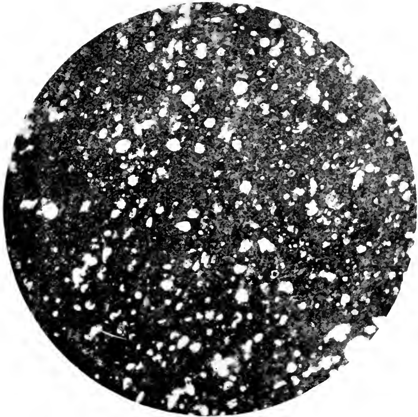
FIG. 8.— Photomicrograph of a typical weathered shale from Fajardo Playa, magnification 28 diameters
