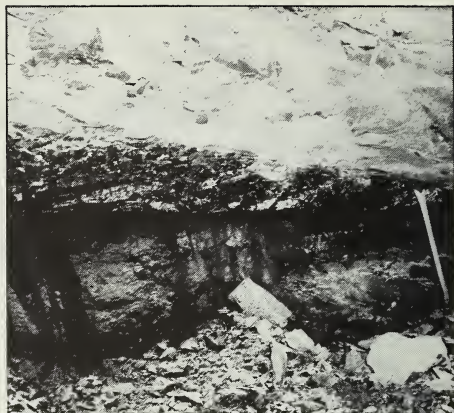
Figure 6 Channels cutting out coal at the abandoned Freeman Crown I Mine. The channel fill is primarily gray silty shale and siltstone; slickensides were caused by uneven compaction.
