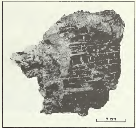
Figure 33 Specimen of Herrin (No. 6) Coal affected by white top. Light-colored clay has infiltrated both vertical and horizontal fissures in the coal without rotating the banding. (Photo from Damberger, 1970.)
