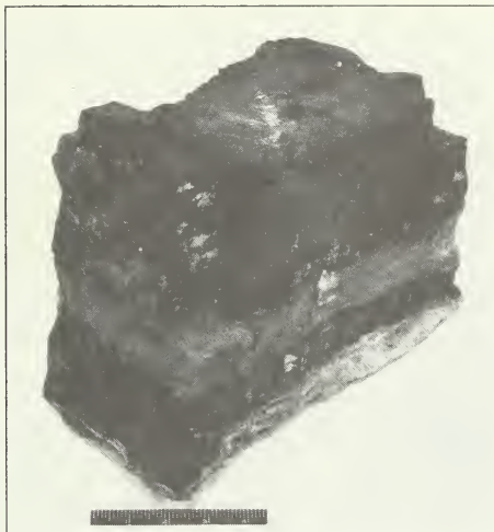
Figure 16 Block of Herrin (No. 6) Coal showing the "blue band" and two well developed sets of cleat at right angles to each other. (Scale in cm.)
