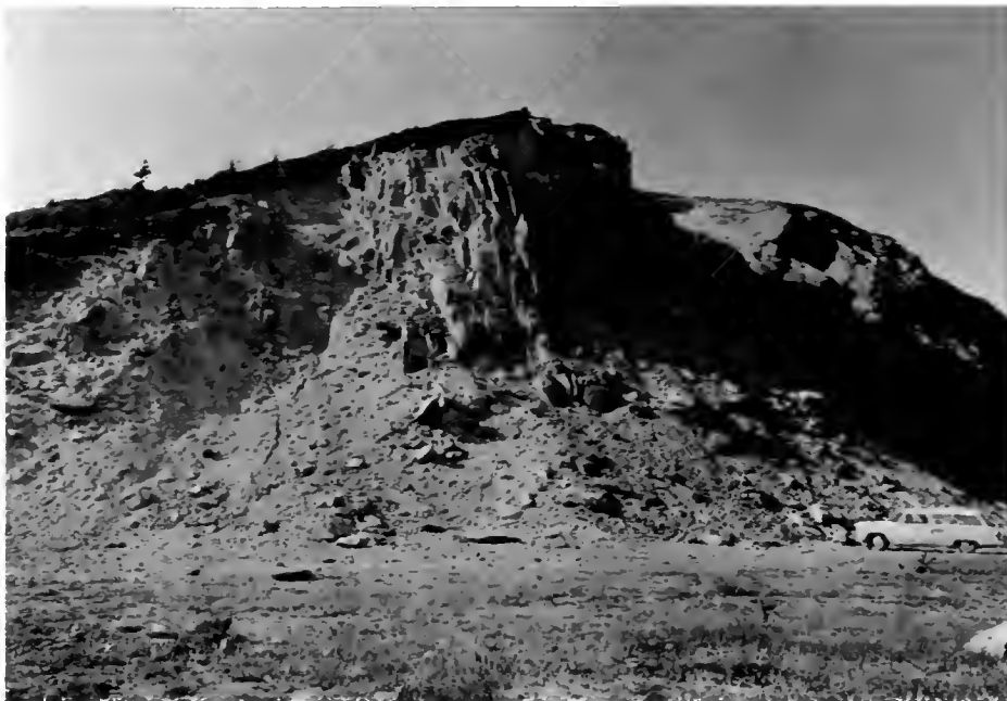
Figure 5. Quarry in small nepheline syenite stock on east end of Blodgett Peak (Stop 5). Jointing along primary flow banding is nearly vertical in center but dips less steeply on right. Nepheline syenite from quarry was used for road rock and jetty rock.
