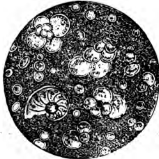
Fig. 94.—Thin Slice or Section of hard White Chalk, examined by transmitted light and highly magnified. Entire shells and fragments of Globigerina and other foraminifera are seen. (After Nicholson.)
