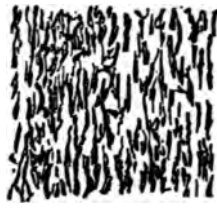
Fig. 90A.—Slate, from Llanberis, in North Wales; the particles of mica all lie parallel to each other; cleavage perfect. (After Sorby.)
