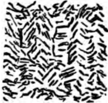
Fig. 90.—Slate, from Shap, the particles of mica lying in all directions; cleavage imperfect. (After Sorby.)
