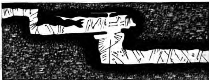
Fig. 78.—"White Rock Trap," or Basalt, traversing the Thick Coal near Rowley, South Staffordshire. The igneous rock is about one foot thick; it has altered the coal—made it dull, friable, and earthy—to a distance of twelve inches.—Scale, five feet to one inch.
