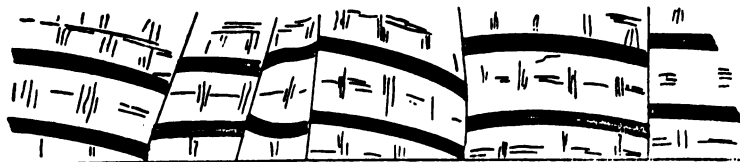
FIG. 11.—Diagram Section of small faults in the Portland Stone, Brill. This dislocation of the beds was seen in a small pit about two-thirds of a mile south-west of the church. The dark bands are two shaly layers; the greatest displacement, or "throw," only amounts to two feet. (After A. H. Green, Geol. Survey.)
