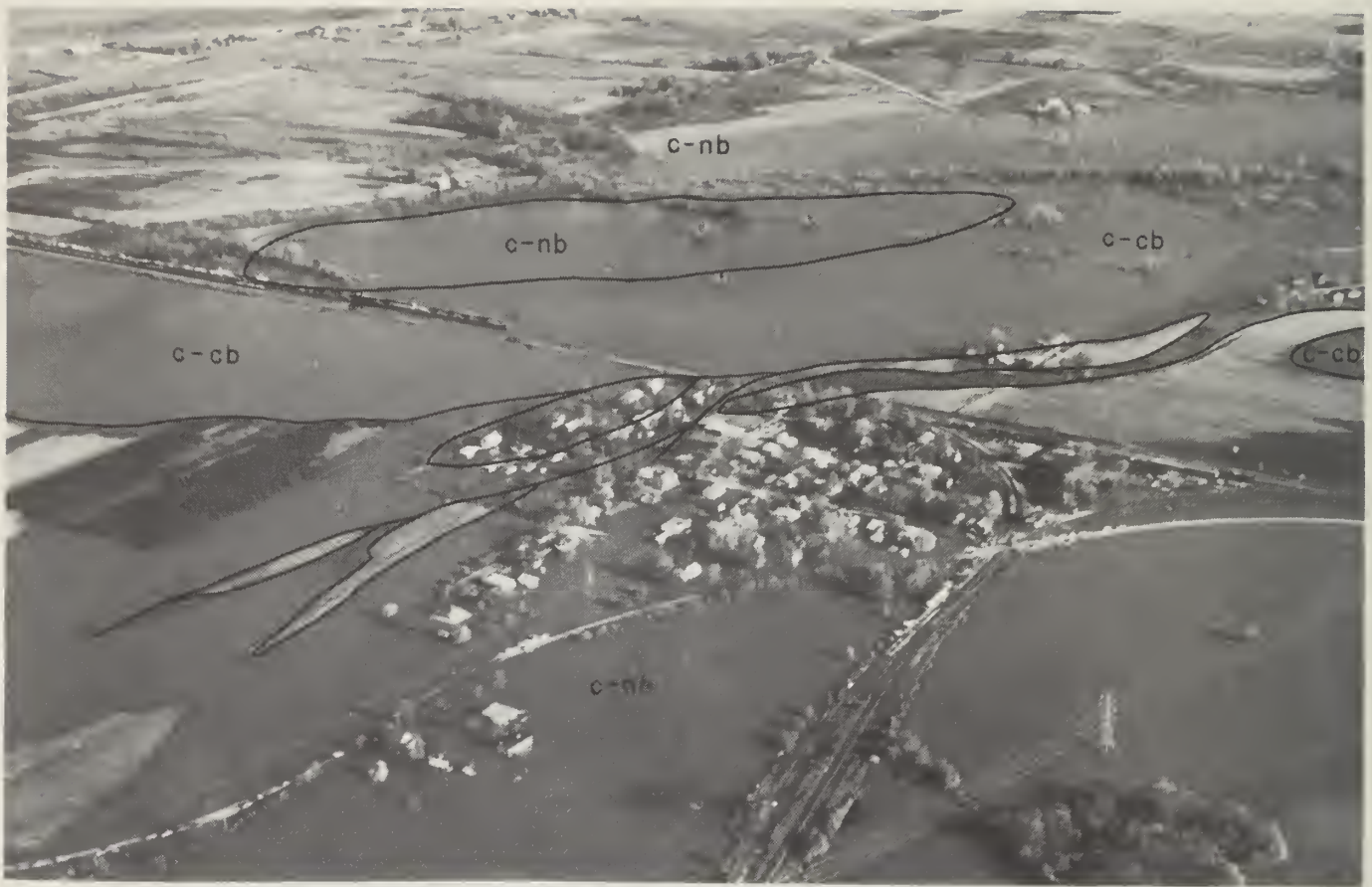
Figure 10. Aerial view of Barstow, looking northwest, April 27, 1973. River bars stand above flood level, whereas abandoned river channels and low areas between bars are inundated. For explanation of symbols see legend of plate 1.
