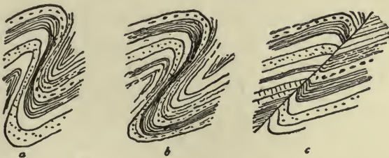
Fig. 101.— Sections to show the relations of Plications (a, b) to reversed Faults (c).
