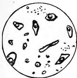
Fig. 68.—Cavities in quartz containing liquids (magnified).
