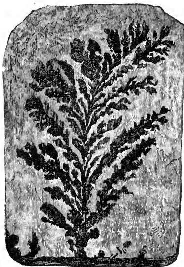
Fig. 55.—Dendritic markings due to arborescent deposit of earthy manganese oxide.
