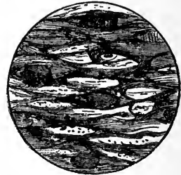
Fig. 104.—Sheared red sandstone forming now a micaceous schist, Keeshorn, Ross-shire (magnified).
