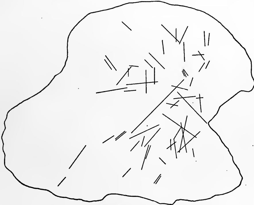
FIG. 10.—Microscopic fractures in granitic quartz.
