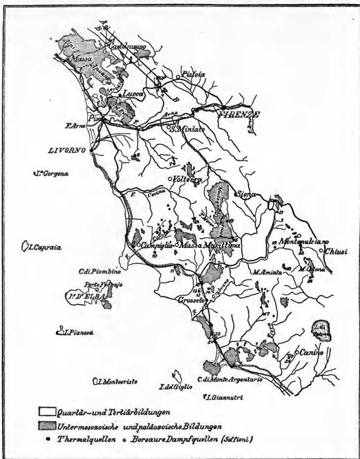
FIG. 102.—Geological sketch map of part of Tuscany, showing the location of hot springs (solid dots .) and Borax Fumaroles or Saffioni (asterisks *). The shaded areas indicate lower Mesozoic and Palaeozoic, the white Tertiary and Quaternary formations. Scale approximately 1:200,000. ( Zeitschr für Prakt. Geologie , 1893, p. 373.)
