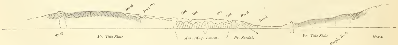
FIG. 17.—Section of the Primal and Gneissic Strata, and of the Auroral Limestone and its Ore-Ground, near Spring Mill.
