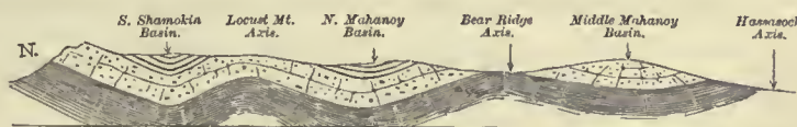
FIG. 230.—Section of East End of the Mahanoy Coal-field. (The S. and middle N. dips are too gentle.)
