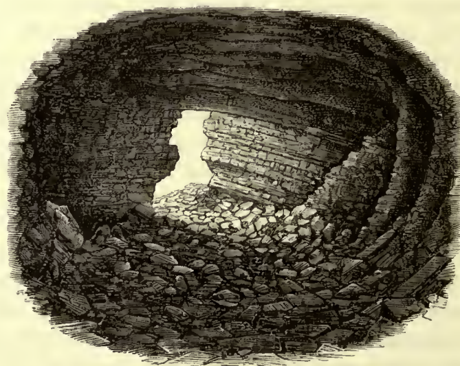
FIG. 223.—One of the Cave Workings in the South Mine of the Great Lehigh Summit Coal Seam: height about 40 feet.
