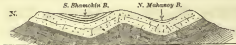
FIG. 226.—Head Mountain, S.W. Side of Lindner's Gap. Note.—The Cut does not represent sufficiently steep dips in the S. Basin.
