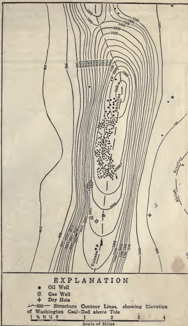
FIG. 26.—Contour map of a part of the Volcano anticline, Wood, Richie, Wirt and Pleasants Counties, West Virginia. Contour interval 100 feet. (After White, Grimsley and Hennen, West Virginia Geol. Survey. )
