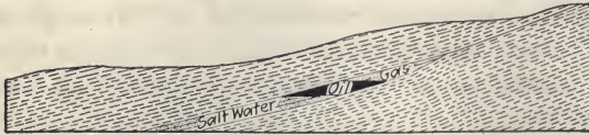
FIG. 45.—Sketch showing reservoir sealed by impervious rocks overlying and underlying the reservoir rock and joining above the reservoir.
