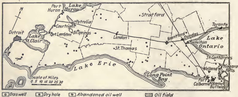
FIG. 189.—Sketch showing location of oil fields and wells in South Ontario. (After Clapp.) The heavy lines indicate lines of sections given in Figs. 190 and 191.
