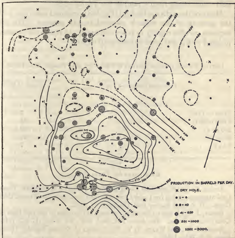
FIG. 153.—Sketch showing the distribution and production of wells, in the Thrall oil field, Texas. Contour lines show position of upper surface of oil-bearing rock in feet below sea level. (After Udden and Bybee.)
