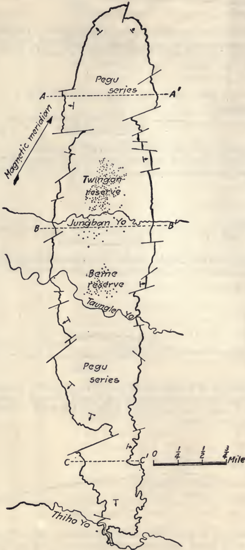
FIG. 38.—Sketch plan of Yenangyaung oil field, Burma. The heavy black line is the red bed at the base of the Irrawadian formation. (After Pascoe.) For sections along AA', BB' and CC', see Fig. 39.
