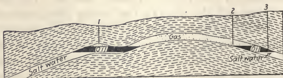
FIG. 79.—Sketch showing gas wells (1 and 2,) that would become oil wells if, because of decrease of pressure of gas, the plane of contact of oil and gas were to rise. If the plane of contact between oil and water were elevated because of removal of gas or oil, well 3 would cease to flow oil and would flow water.
