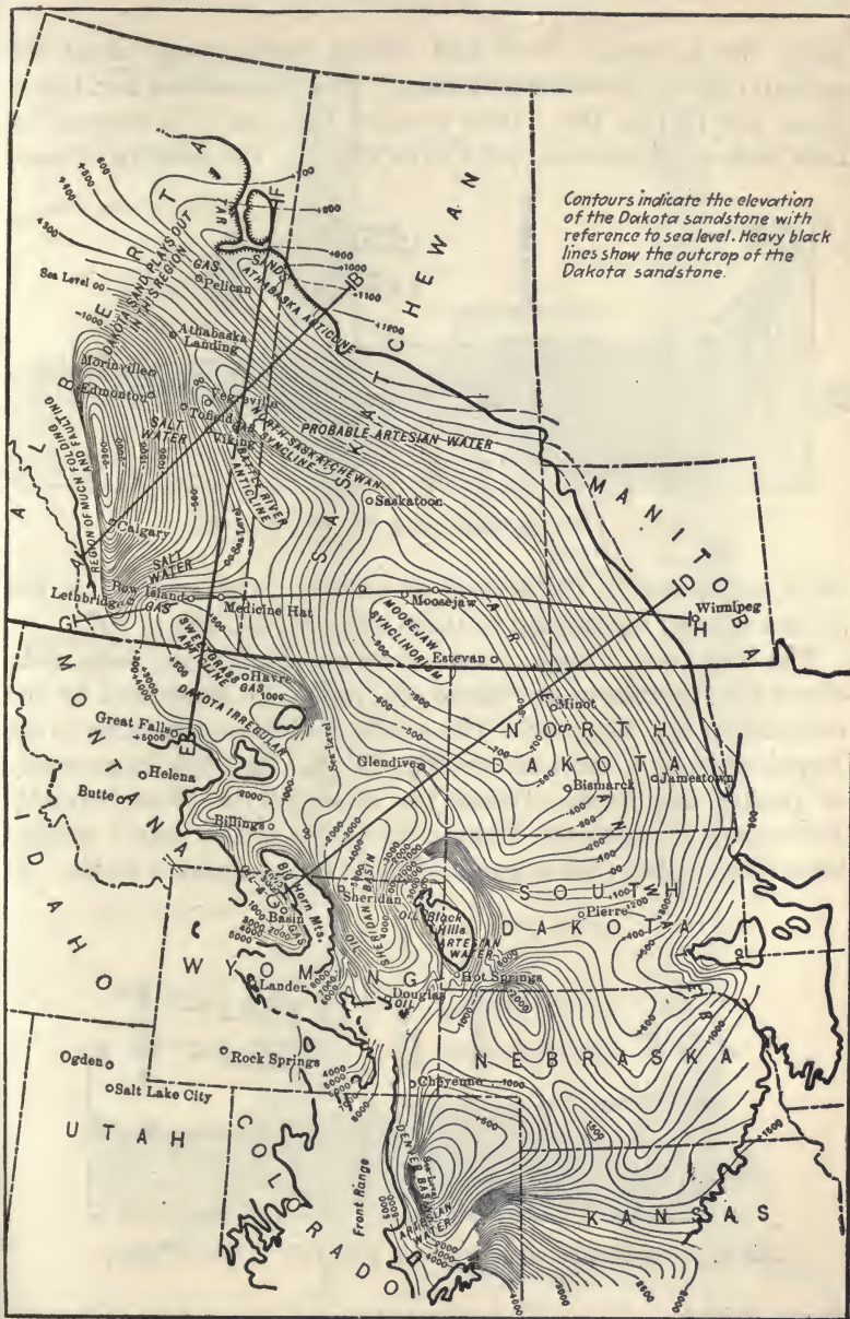
FIG. 193.—Map showing generalized structure of the Dakota sandstone in the United States and Canada east of the Rocky Mountains, with relation to the oil, gas, and water reservoirs. Sections along lines A-B, etc., are given on Figs. 194-197. (After Huntley.)
