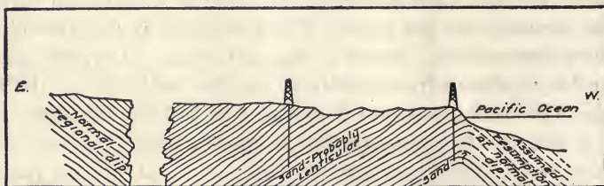
FIG. 254.—Generalized geological section, showing structure of Negritos oil field, Peru (looking south.) The western part of section is hypothetical.
