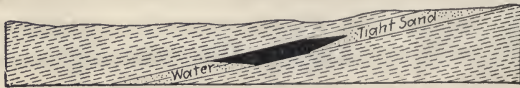
FIG. 47.—Sketch showing reservoir sealed by tight sand. Black is oil and gas.
