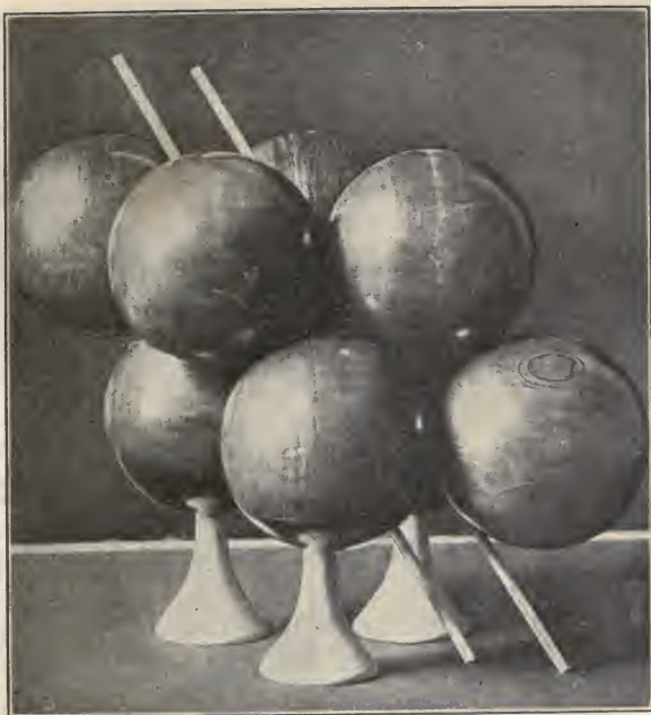
FIG. 8.—Spheres packed in the most compact manner possible. The face angles are 60^\circ and 120^\circ . (After Slichter.)
