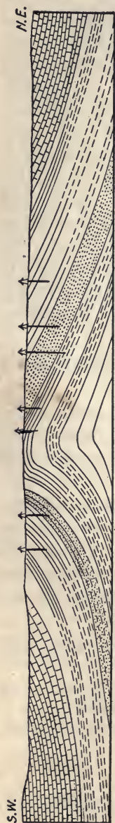
Fig. 32.—Section of western part of the Balakhany oil field and part of Zabrat oil field near Baku, Russia. (After Barbot de Marini.)
