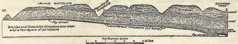
FIG. 105.—Cross-section from Irving to Campton, Kentucky, showing the dip and thickening of formations to the east, the structural features on which oil and gas are found and the general attitude of the surface. (After Shaw.)
