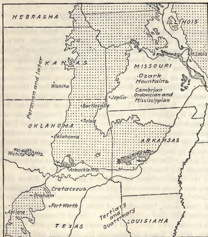
FIG. 118.—Sketch map showing geology of region containing Mid-continent oil field. The Pennsylvanian outcrops in the areas shown by dots, widely spaced. There are small outcrops of Silurian and Devonian rocks in the Ozark region. These are not shown in the sketch. The igneous rocks which are in the areas represented by small crosses, are older than the sedimentary rocks.
