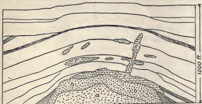
FIG. 42.—Section of Spindletop oil field, Texas. a , rock salt; b , gypsum; c , limestone. (After Lee Hager.)
