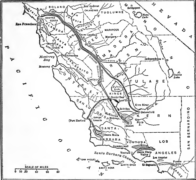
FIG. 177.—Map of part of California, showing oil districts and pipe lines. (After Arnold and Garjias.)
