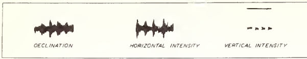
FIG. 141—BEAT-RESPONSES OF VARIOMETERS FOR INTERMITTENT SINUSOIDAL FIELDS OF ONE-HALF MINUTE DURATION APPEARING AT SUCCESSIVE THREE-MINUTE INTERVALS, O, H, AND Z
