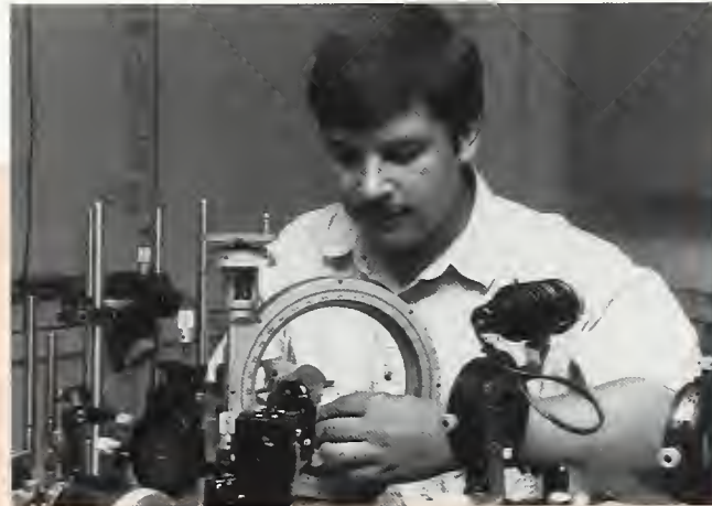
To measure various properties of mantle minerals, Sinogeikin positions samples on the Brillouin system.
