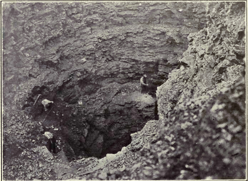
Fig. 5.—View from Top of Glory-hole. The Material is Loosened and Rolls down before the Closed Sliding Door.
