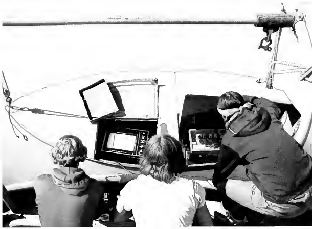
Researchers ready depth-recording instruments inside Bergy-bit's covered hull (top). Glaciologist Austin Post (middle) plots bathymetric contours aboard Growler. Bergy-bit's chart (bottom) shows the Gilman Glacier ice front. On the author's trip aboard Growler, Bergy-bit charted an underwater canyon at the Johns Hopkins Glacier ice front.
