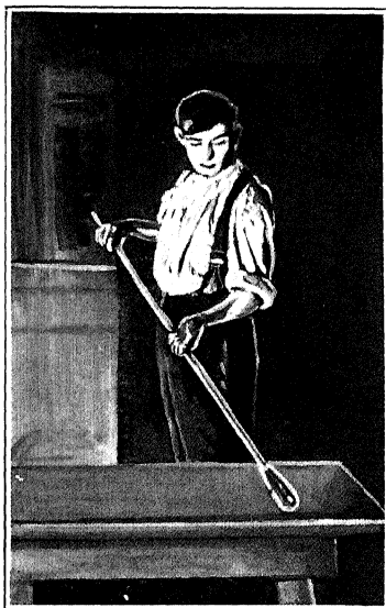
Figure 4. Rolling Glass on Marver
