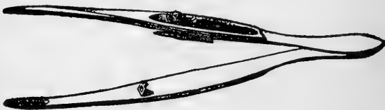
FORCEPS FOR LIFTING BLEEDING AND WOUNDED BLOOD VESSELS SO THAT THEY MAY BE TIED.
