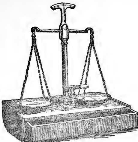
BALANCE WEIGHING ONE GRAIN TO A FEW OUNCES.
