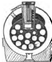
Fig. 1. Section of Boxer Shrapnel Shell with fuze. Diaphragm.
