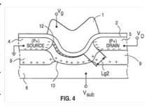
than in a conventional MOSFET. *See* 4:3-8 ("By comparing Fig. 4 to Fig. 9, it can be seen that . . . the distance Lg2 between the end of channel region 12 and the drain 5 is longer than the distance Lg1 indicated in Fig. 9.").
