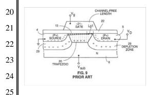
are the source (labeled "4" in Fig. 9), where current enters the transistor; the drain (5), where the current leaves the transistor; and the gate (21), which starts and stops the flow of current. When the transistor is turned on, current flows from the source to the drain through a channel (13). When the voltage is
