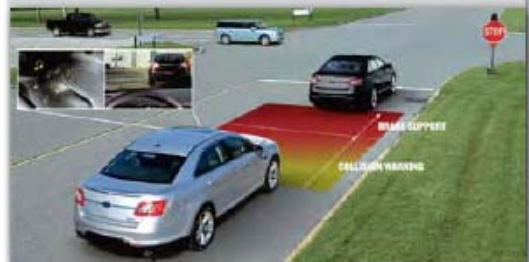
Ford’s Adaptive Cruise Control and Collision Warning with Brake Support allows drivers to set the vehicle’s speed and maintain it without using the accelerator pedal, using radar sensors to detect moving vehicles ahead and warn drivers of collision risks.
