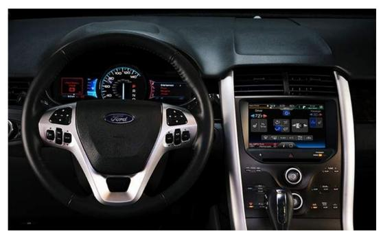
209. The primary centerpiece of MyFord Touch is an eight-inch LCD touchscreen that is located in the center stack, depicted in the photograph below.
