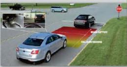
Ford's Adaptive Cruise Control and Collision Warning with Brake Support allows drivers to set the vehicle's speed and maintain it without using the accelerator pedal, using radar sensors to detact moving vehicles ahead and warn drivers of collision risks.
