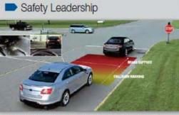
Ford's Adaptive Cruise Control and Collision Warning with Brake Support allows drivers to set the vehicle's speed and maintain it without using the accelerator pedal, using radar sensors to detact moving vehicles ahead and warn drivers of collision risks.
