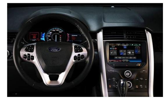
209. The primary centerpiece of MyFord Touch is an eight-inch LCD touchscreen that is located in the center stack, depicted in the photograph below.
