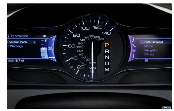
212. These two additional interfaces are not touchscreens. Rather, the user navigates these through a five-way control located on the steering wheel (images of the controls on the steering wheel are contained in the image in paragraph 227 above). They allow the user to perform some of the same functions that can be performed on the center stack interface, however, on a more limited basis.
