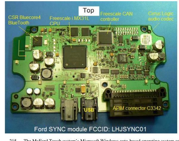
215. The MyFord Touch system's Microsoft Windows auto-based operating system can also receive software updates through the use of the Class Vehicles' USB ports.
