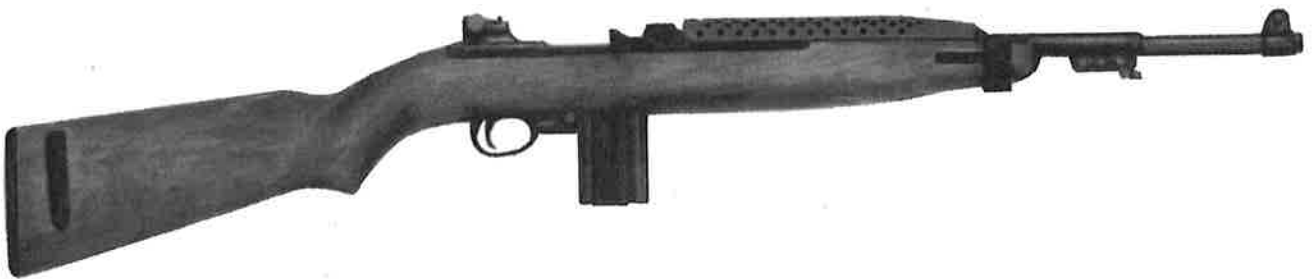
The M1 carbine in many ways served as the yardstick against which the AR-15 was measured. Like the AR-15, the M1 carbine was light and handy, firing a cartridge that produced little recoil and was easy to manage during automatic fire.
