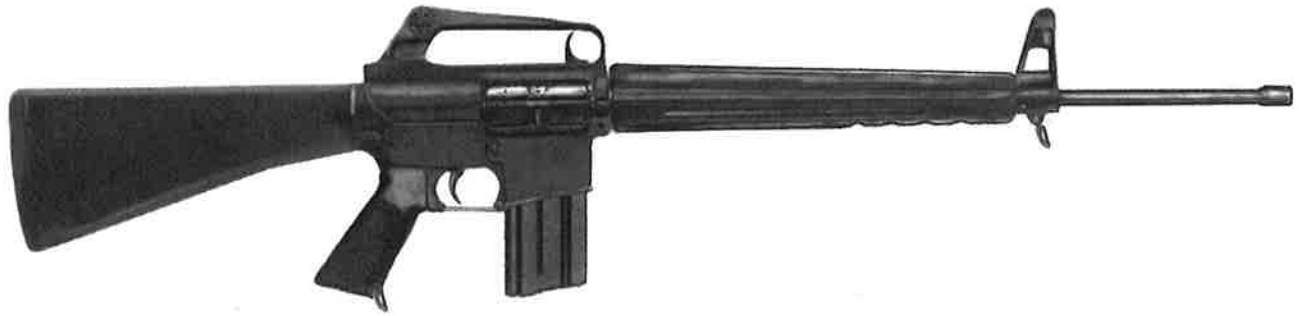
Early AR-15, identifiable by its lack of flash hider.
