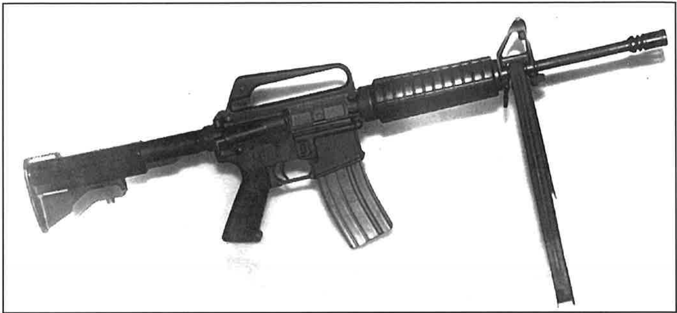
A right-side view of the Colt Model 653 carbine. The buttstock is in the maximum extended position and the weapon is loaded with a production 30 round magazine. The forward bolt assist can be seen on the upper receiver just above the pistol grip. The spring-loaded ejection port is closed in this picture. The weapon is supported by an M3 bipod clamped below the front sight and the muzzle is mounted with the third model "birdcage" flash suppressor.
