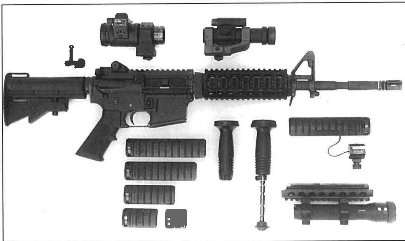
The complete Knight Armaments Company (KAC) Modular Weapon System recently adopted by the Special Operations Command (SOCOM) for issue to their forces including the Navy SEALs as the M4A1 carbine. The basic weapon is the Colt Model R0927 carbine version of the M16A2 rifle with the KAC Rail Interface System (RIS) in place of the standard front handguard. The RIS has four MIL-STD-1913 mounting rails that will accept a wide range of accessories for both aiming or controlling the weapon. Accessories in this photo include (above the weapon from left to right) the KAC low-profile folding 300 meter rear sight, the ITT "pocketscope" night vision device on a KAC mount, and the Aimpoint 5000 also on a KAC mount. Below the weapon from left to right are; the five different lengths of handguard sections that can fit on the RIS forend different lengths filling in for the space remaining from various devices, the KAC basic vertical foregrip, the KAC monopod vertical foregrip assembly with the monopod extended. Directly below the barrel is the Leupold visible laser aiming device with its companion panel switch module. Below the Leupold assembly is the tactical Streamlight poly flashlight package held to the mounting plate with KAC rings. In addition to these devices, a folding bipod assembly is also available to go on the RIS-equipped M4A1 carbine PHOTO CREDIT: KNIGHT ARMAMENT COMPANY
