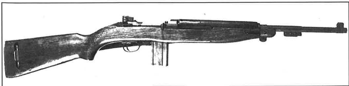
The M2 carbine loaded with a 15 round magazine. The top knob of the small selector lever can be seen at the top of the receiver, above the magazine and just forward of the curved grip of the operating rod.
