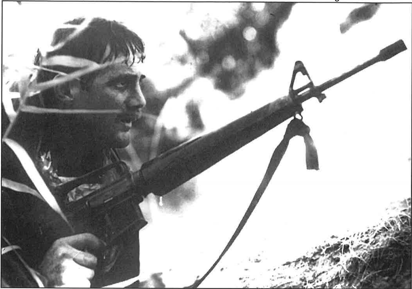
This combat swimmer has just left the water with his Mark 4 variation of the M16A1 rifle. Besides the normal protection from the water that is part of the Mark 4 conversion, this weapon also has a plastic muzzle cap over the flash hider to help keep water out of the barrel. The muzzle cap is plastic and can be easily fired through without any damage to the weapon.
