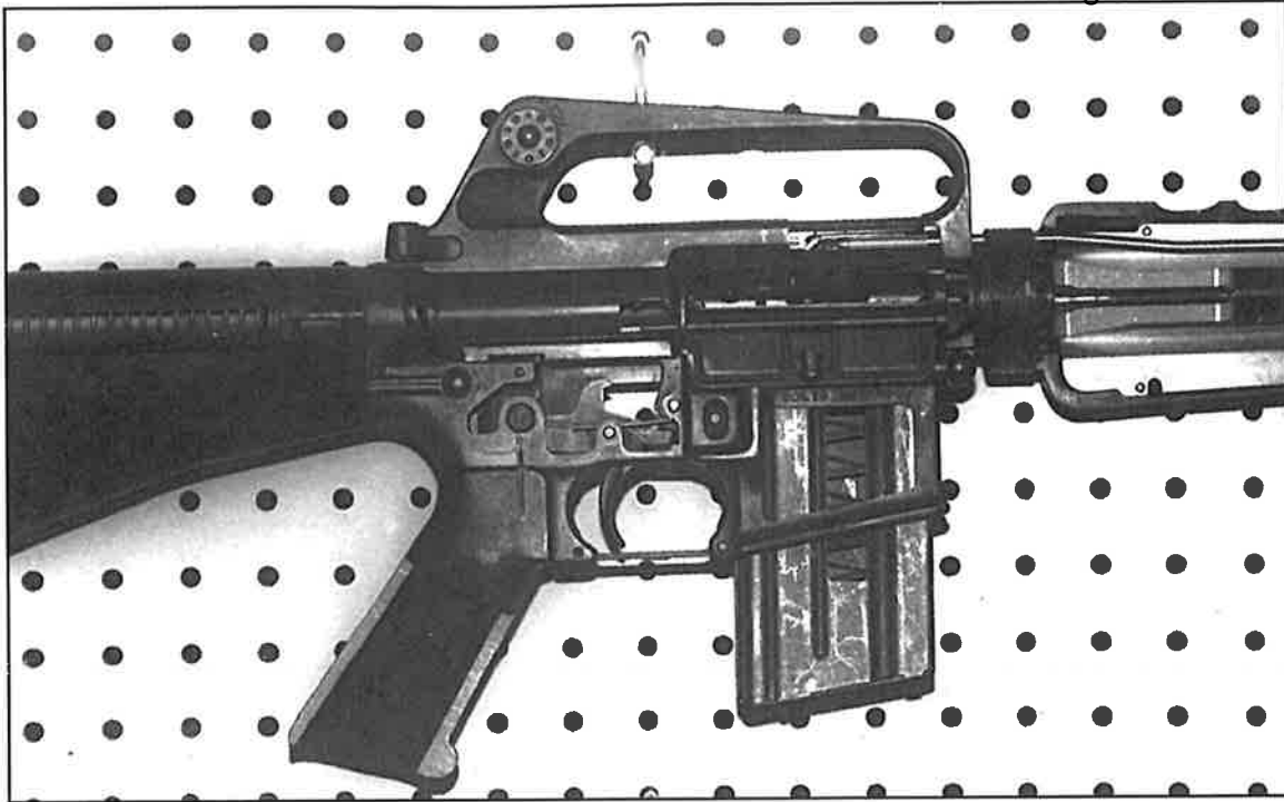
A rare cutaway AR-15 rifle from the Colt Gun Room. This photo shows all of the major internal workings of the AR-15/M16 weapon system. The hammer is forward in the uncocked (fired) position. PHOTO CREDIT: KEVIN DOCKERY/KNIGHT ARMAMENT COMPANY
