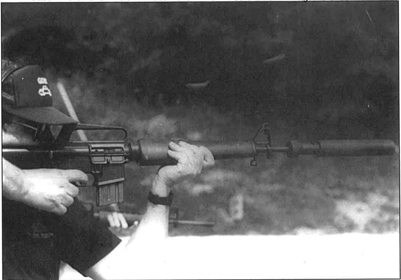
The author firing an M16A1 rifle with a Mark 2 Blast Suppressor mounted on the muzzle. The weapon is firing a short burst on full automatic, two ejected cartridge cases visible as the elongated blurs above the firer's left hand and the weapon's front sight. It is interesting to note the lack of muzzle climb on the weapon, even when fired on full automatic. This lack of rise is a by-product of having the extra weight of the suppressor on the muzzle. PHOTO CREDIT: KEVIN DOCKERY
