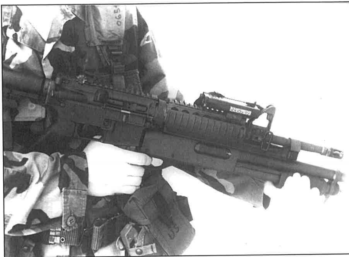
The M4A1 carbine with the Knight RIS system. Mounted on the top rail of the RIS forend is an infrared aiming light. On either side of the forend are "11 rib" full length handguard sections. On the bottom of the RIS, held in a firing position by the operator, is the KAC "Masterkey" shotgun, a modified 12 gage Remington 870 pump shotgun used primarily for opening doors by blasting off the hinges/lock. PHOTO CREDIT: KNIGHT ARMAMENT COMPANY
