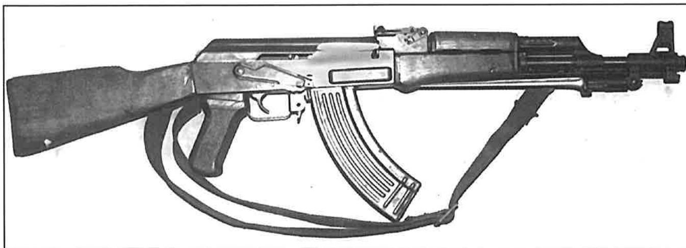
A right-side view of a late-model Chinese Type 56 rifle with a folding, spike bayonet. This is the Chicom version of the Soviet AK-47 and was the most common weapon of its type encountered by the SEALs in Vietnam.
