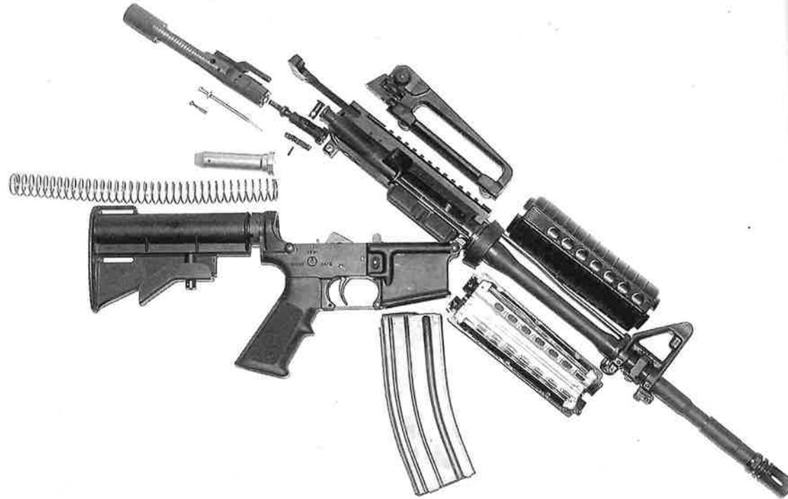
103. Right side view of the M4 carbine, shown partially disassembled.
