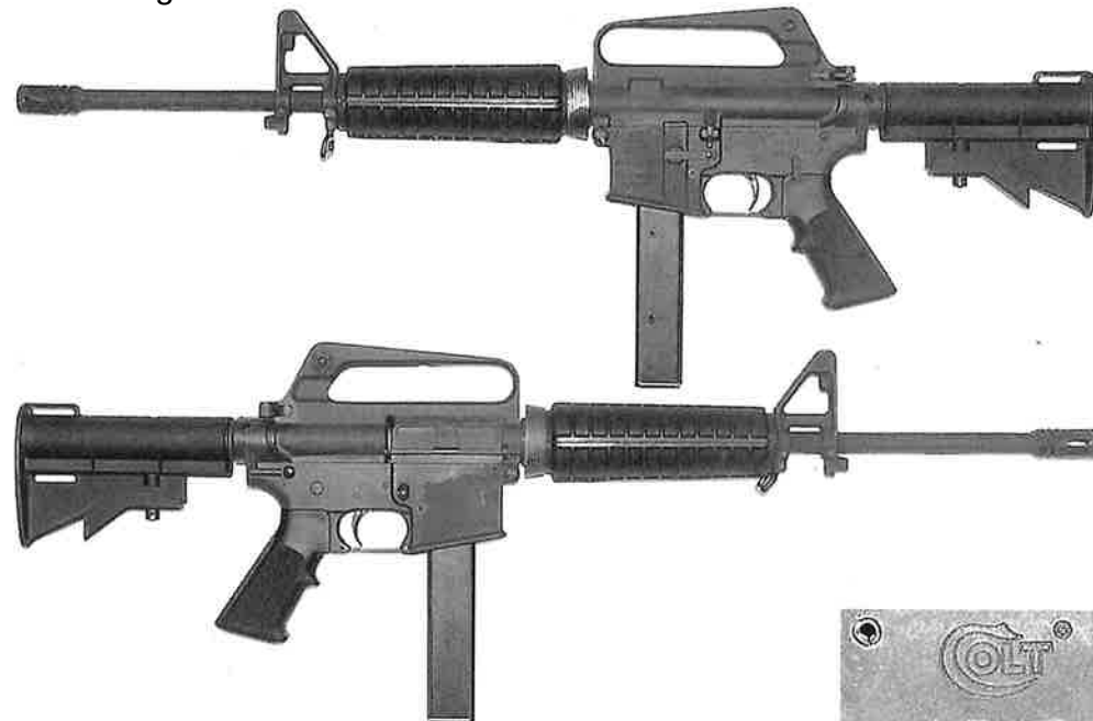
366. Left and right side views of the original version of the Colt AR-15 9mm Carbine, with 16" barrel.
