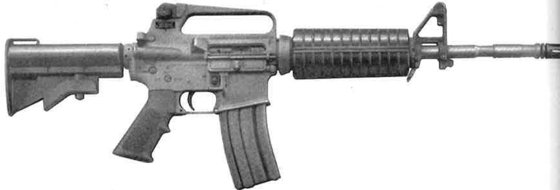
79. Right side view of the XM4 carbine, the experimental version of the M4.
