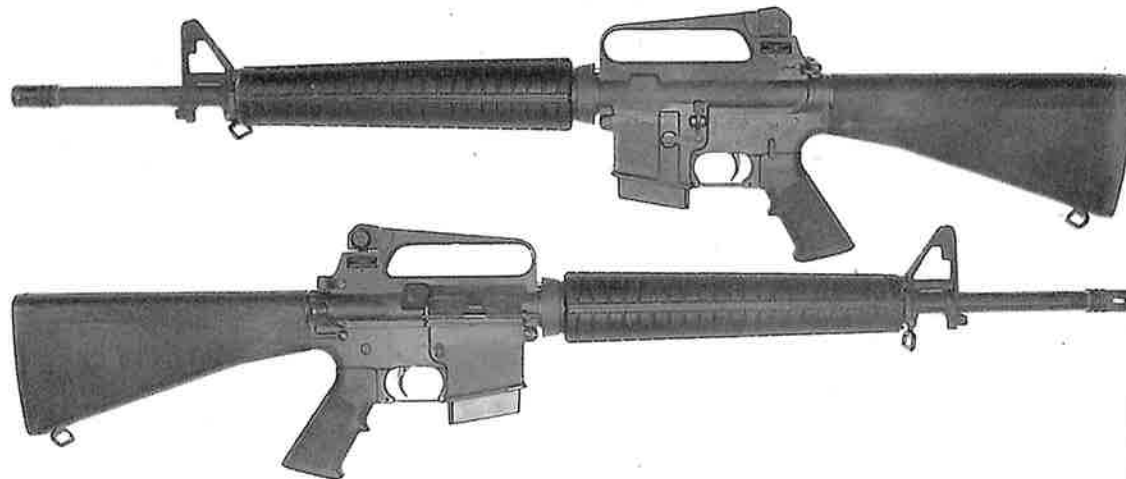
372. Left and right side views of the AR-15A2 Government Rifle, which was identical to the Match HBAR, minus the heavy barrel.
