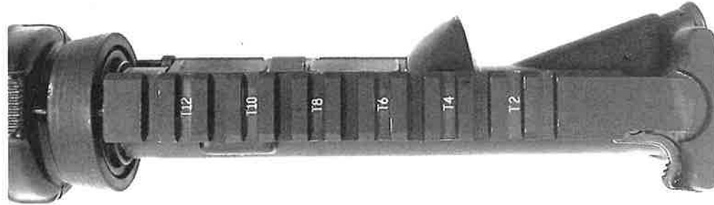
95. Top view of an M4 carbine, showing the integral MIL-STD-1913 rail.
