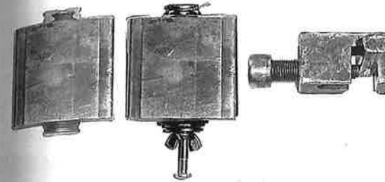
29. The two halves of the magazine well brace, left, and the "A2" punch and its positioning fixture.
