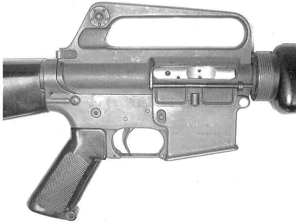
350. Right side closeup of the original semi-automatic-only pilot model, serial no GX 4968. The faint two-line hand-stamped marking on the magazine well reads "Colt Gun Room".
