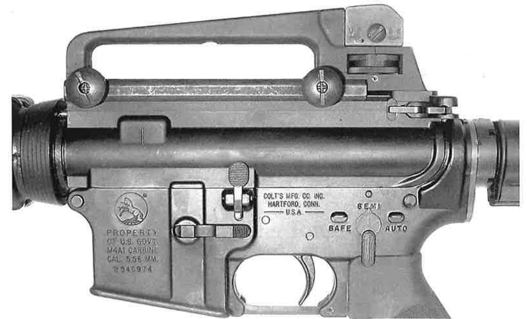
102. Left side closeup of the Colt M4A1 carbine, showing markings. Note the AUTO selector lever setting. ©2003 by Colt Defense LLC. Used with permission, all rights reserved
