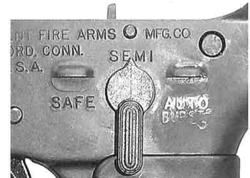
33. Left side closeup of an upgraded early rifle, showing the "AUTO" marking Xed out and replaced with "BURST".
