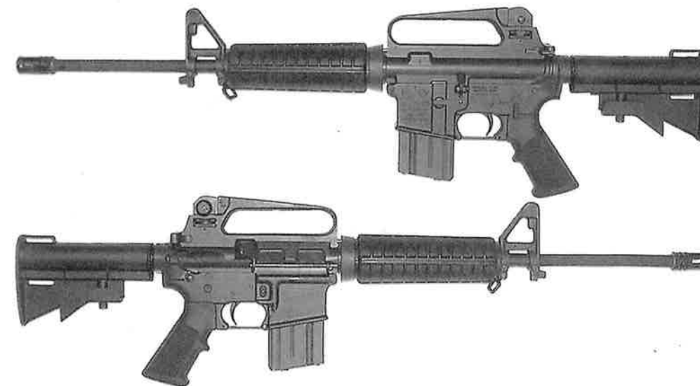
374. Left and right side views of the Colt AR-15A2 Government Carbine (Model R6520), fitted with the fully adjustable M16A2 rear sight and the integral spent cartridge case deflector.
