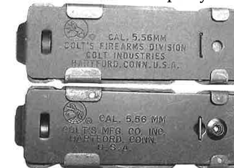
409. Underside views of two magazine floorplates. Above: early commercial five-round magazine with no rivet in removable floorplate. Below: later five-round magazine with permanent rivet in floorplate.
