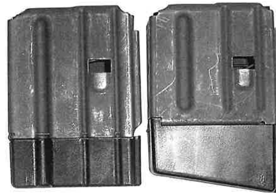
410. Left side views of the two post-assault weapon ban restricted capacity Colt AR-15 magazines. Left: eight-shot, with grooved, flat-bottomed polymer base cap. Right: nine-shot, with plain, angled-bottom polymer base cap.
