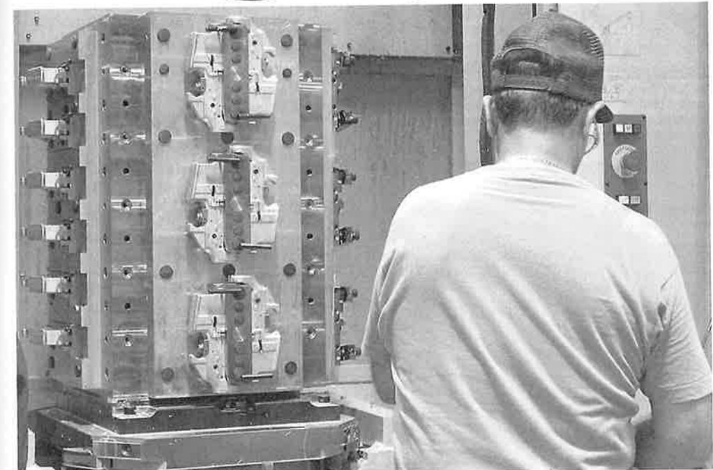
14. Lower receiver manufacturing at Colt Defense, LLC is done on state-of-the-art TOYODA horizontal machining centers, equipped with pallet changers. There are 24 for-
