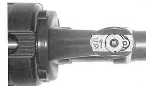
8. Top closeup of the new M16A2 four-position square front sight post.
