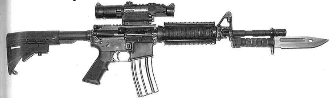
106. Right side view of an M4A1 carbine fitted with the Leupold Mark 4 CQ/T scope, Knight's Armament RAS, both discussed in Chapter Thirteen, and M9 bayonet.
