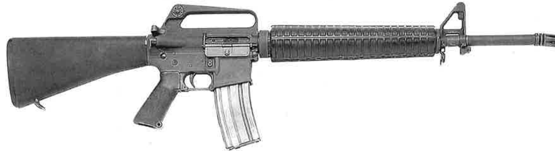
1. Right side view of the early experimental M16A1E1. This image originally appeared in TBR as fig. 369. Note the A1-style rear sight, stock and pistol grip. The
