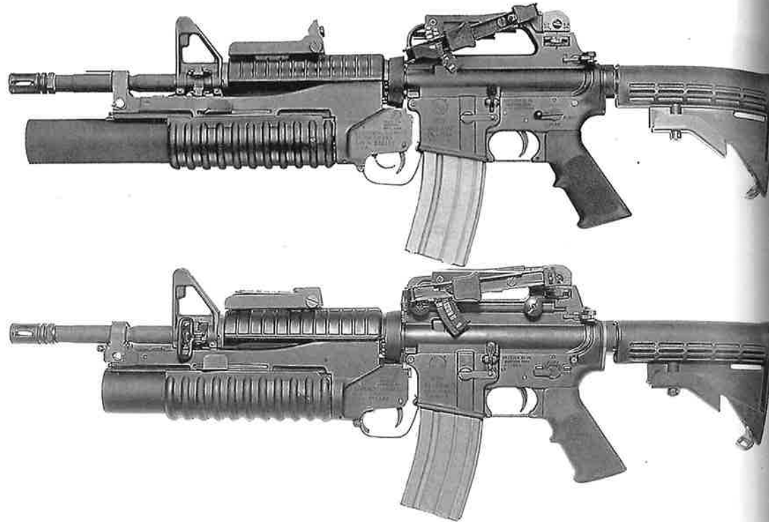
107. Left side views of two Colt carbines, showing the two versions of the M203 grenade launcher offered by Colt. Above: Enhanced M4 (with four-way fire control setting), fitted with the standard-length M203. Below: M4A1 (with AUTO fire control setting), fitted with the shorter 9" carbine version of the M203. ©2003 by Colt Defense LLC. Used with permission, all rights reserved
