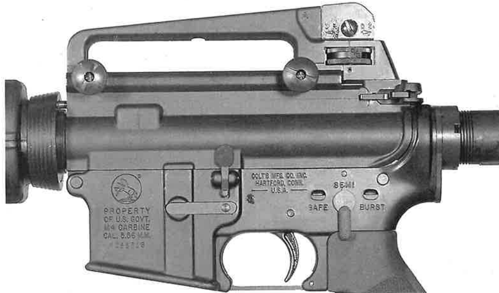
100. Left side closeup of a US government-issue M4 carbine with the detachable carrying handle installed, showing markings. Note the markings on the elevation knob, "6/3", which differ from the standard M16A2 rifle sight which is marked
